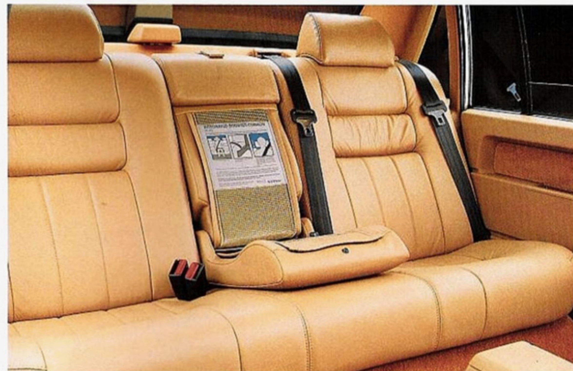
A child's booster cushion is built into the rear seat. Head restraints and 3-point seat belts in all three seating positions are also standard.
