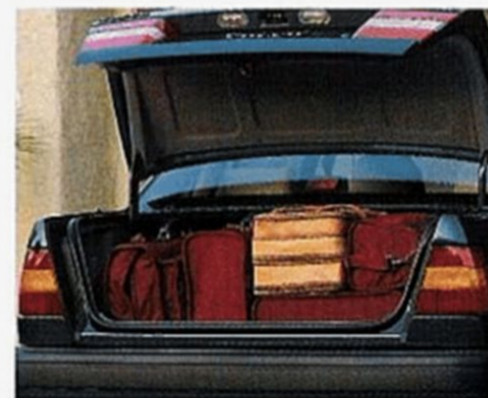
The 16.6 cubic-foot capacity (0.47 cubic meters) and low liftover height make the trunk easy to use.
