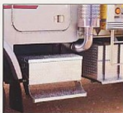
The battery box can be mounted under the steps, where access is quick and easy.
