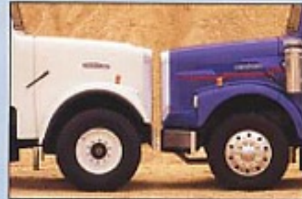
Choose set-forward or set-back front axle to match your maneuverability and weight distribution requirements.
