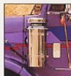
The high capacity of our optional cowl-mounted air cleaners assures full power in dusty conditions.
