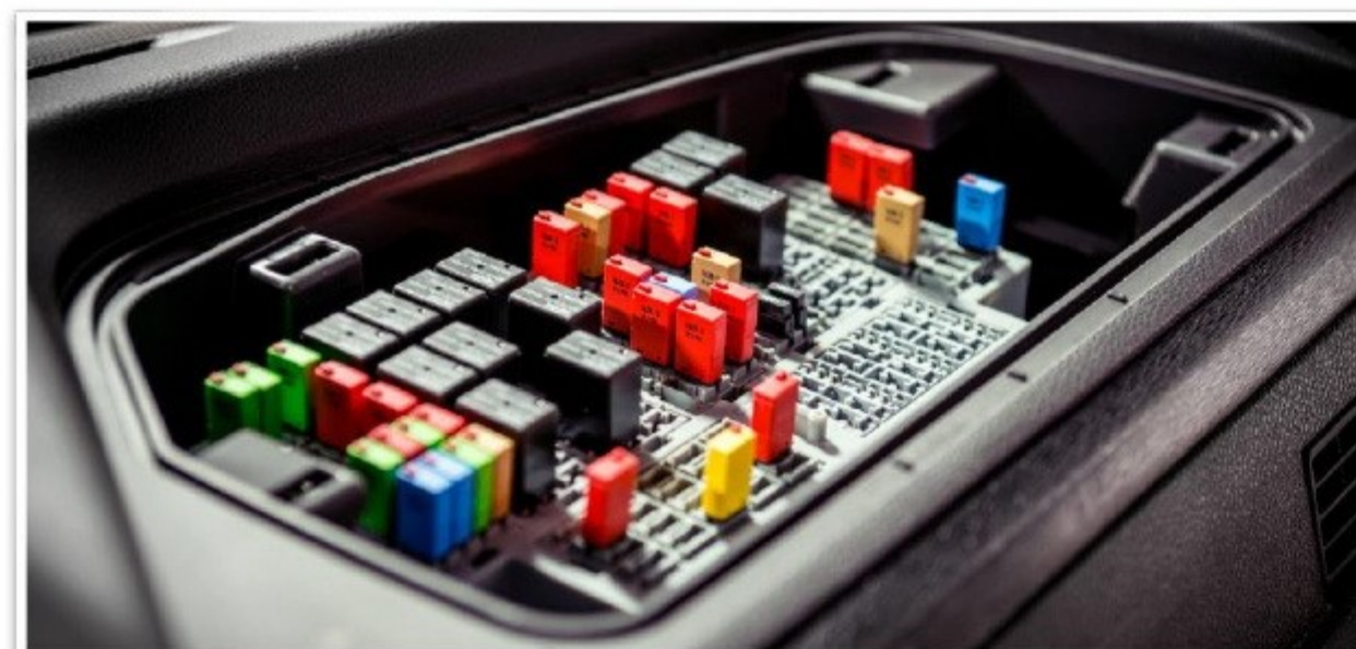
In-cab electrical panel
