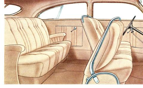
Rear compartment is readily accessible through two wide doors by tilting the back of the front seat forward. Seat is not divided and accommodates three.
