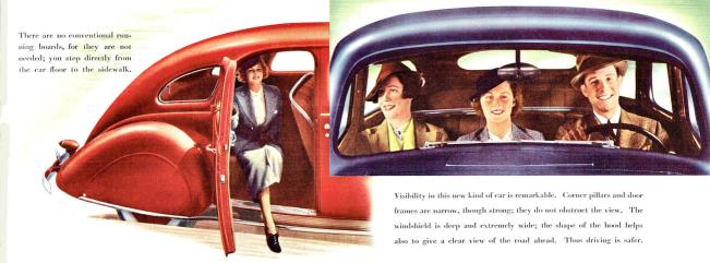
The unique body design gives, owners declare, the most thrilling ride on the roads! Body and frame are one, in the LINCOLN-ZEPHYR, welded together. Around this framework—strong and rigid—steel paneling is welded on top, sides, bottom. You ride surrounded by steel and close to the ground.
