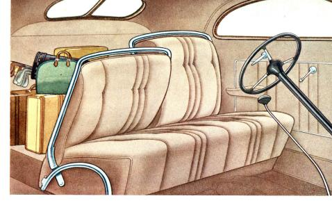
A new Lincoln-Zephyr body type for 1937. Both sides of the divided scat-back tilt forward providing convenient access to the large luggage space behind the scat,
