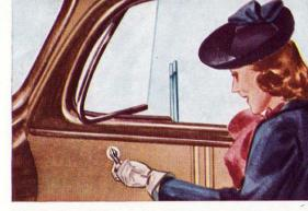
The Ford ventilating system gives you complete control of air circulation. In closed types, metal divider strip slides down with rear half of window. Super De Luxe Ford has crank control for the ventilating wing.
