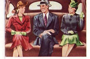
Built for big people, the 1941 Fordor has a front seating width of 56". Rear compartment is 57" wall to wall, with 52" between arm rests. The body extends over the running boards to gain extra width inside.
