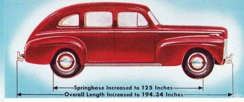
The increased length of the 1941 Ford contributes to its remarkable riding comfort. Springbase has been lengthened in proportion to the new longer wheelbase. Passengers are carried well ahead of the rear axle and spring, near the center of the car where the riding is best. And beneath the flowing beauty of this big car is a rigid new frame, twice as resistant to twisting force as the former rugged Ford frame.
