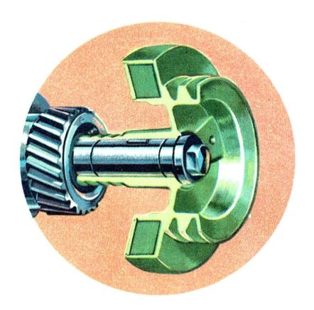
THIS FLUID VIBRATION DAMPER mounts on the front end of the crankshaft . . . absorbs any torsional vibration which might develop at high speed . . . adds a final touch of smoothness. The damper consists of a heavy metal ring (or flywheel); a stable, high-viscosity fluid in which the ring floats; and a welded, hermetically sealed housing. The damper is efficient at all car speeds, is practically unaffected by temperature changes, and never requires servicing.
