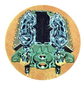
**FULL-FLOW COOLING**—Two high-capacity water pumps, one in each bank of cylinders, circulate water at high velocity around and past *every* cylinder *all* the way through the block . . . then on through the cylinder heads around every combustion chamber to the radiator. Completely water-jacketed valve seats and other parts are all uniformly cooled. A pressure radiator cap keeps system under slight pressure and prevents loss of coolant by evaporation.
