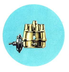
**NEW AUTOMATIC SPARK CONTROL**—The new Lincoln automatic spark control is of the vacuum or differential pressure type. It uses a differential pressure produced within the carburetor, which is a function of speed and load conditions. Accurate and efficient spark control is obtained over the whole engine performance range. Governor weights, used in conventional spark control systems, are eliminated. Construction is simplified and service life is improved.
