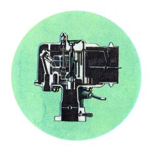
THIS DUAL "CONCENTRIC FLOAT" CARBURETOR is efficient at all engine speeds, road angles, and temperatures (starts in less than two seconds at zero temperatures!). Intake air circulates completely around the fuel chamber . . . keeps fuel comparatively cool . . . minimizes vapor lock and other hot starting troubles. The carburetor includes an automatic "fast idle" control and automatic choke. The latter has a unique filtered-air supply for reliable operation at all times.
