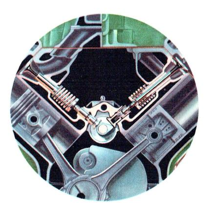
**THIS VALVE SYSTEM** is unusually quiet, efficient, and durable. It consists of zero-clearance, hydraulic valve lifters that eliminate tappet noise and assure full seating . . . exceptionally large-diameter, non-vibrating valve springs . . . hardened alloy-steel valve-seat inserts for the exhaust valves . . . one-piece valve guides pressed in block for rapid heat transfer and low valve temperatures . . . and completely water-jacketed valve seats.
