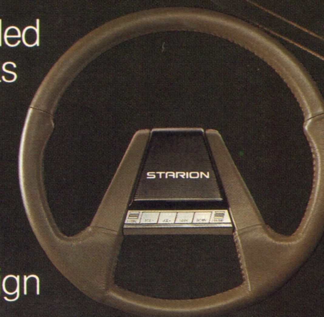
Starion LE model includes remote radio switches mounted right in the steering wheel for convenient control.
