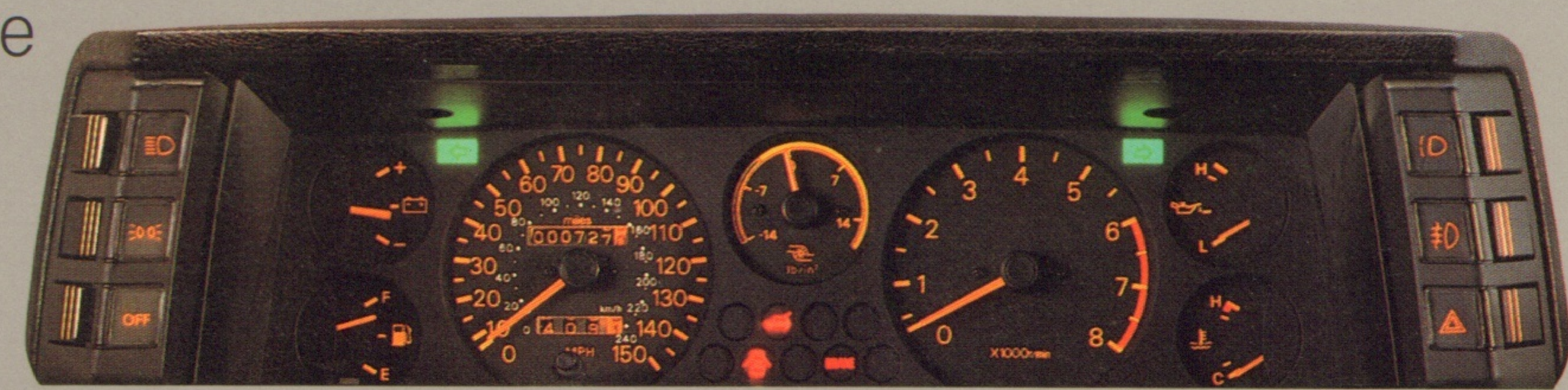
Full analog instrumentation includes a turbo boost gauge. It's logically situated and easily visible, so you can get all the Starion's vital information at a glance.
