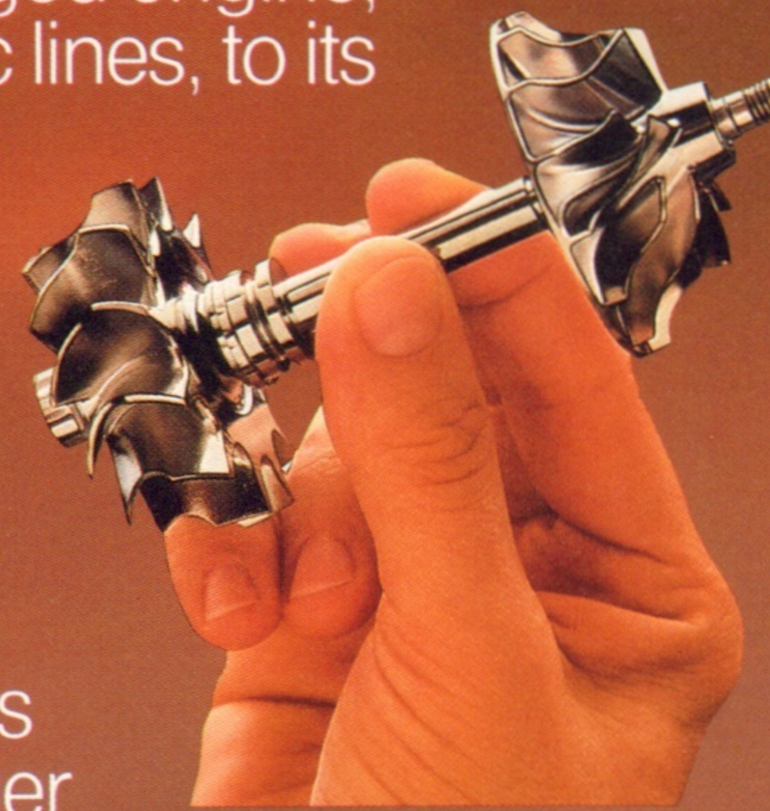
A responsive 8-oz. turbine assembly virtually eliminates turbo lag.
