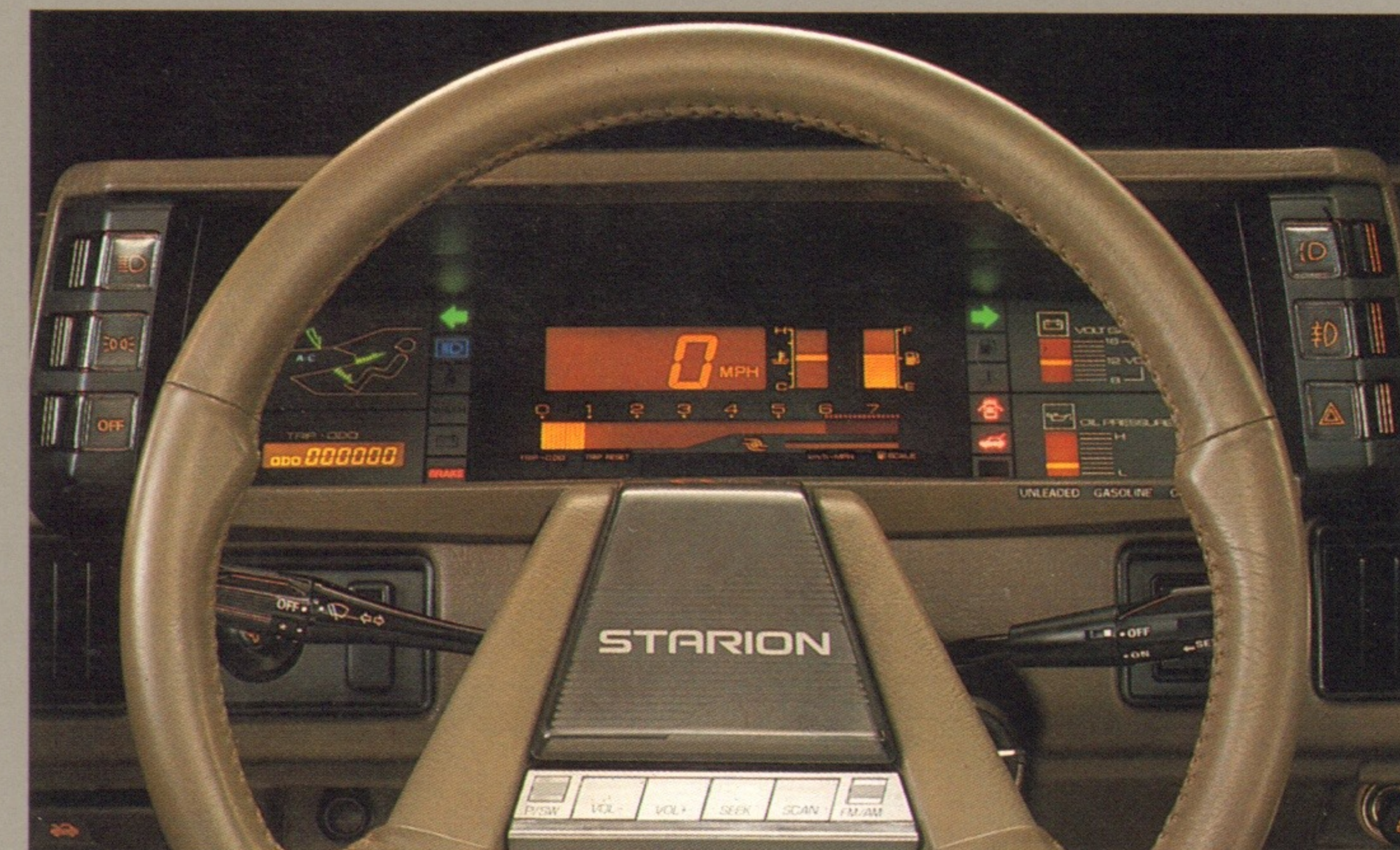
Starion LE model features easy-to-read LCD digital/graphic instruments.
