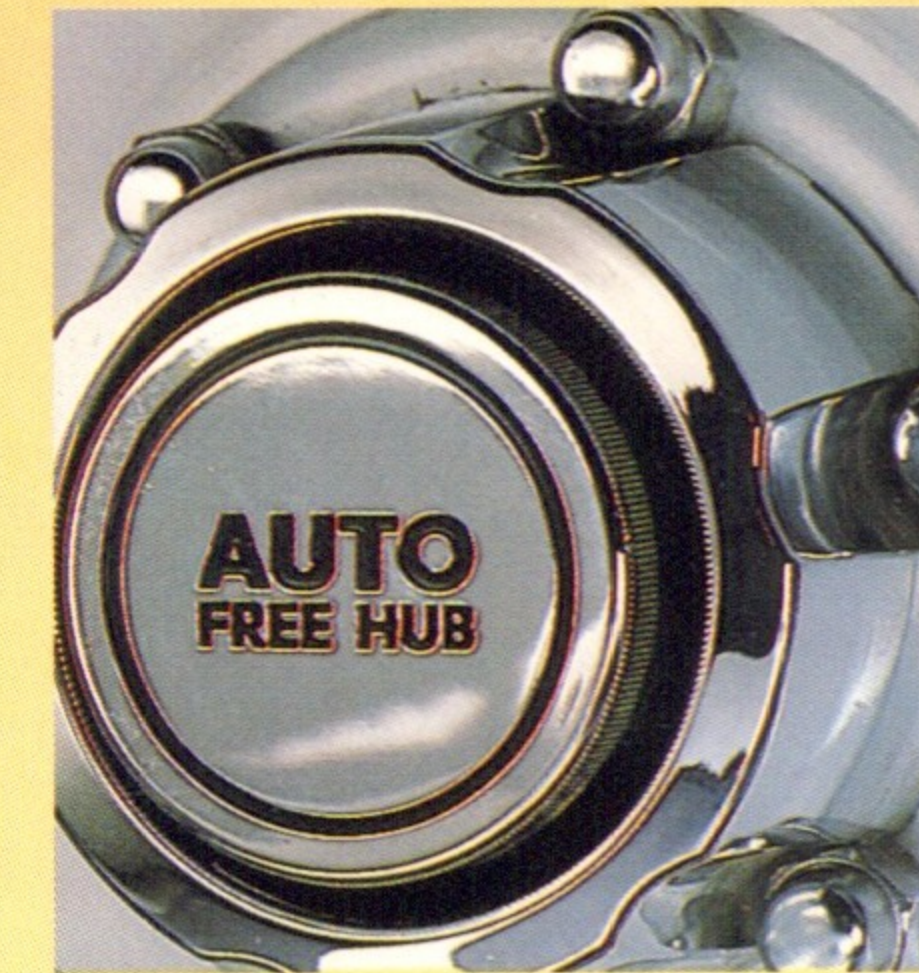
Automatic locking hubs let you go in and out of four-wheel drive without leaving your seat.
