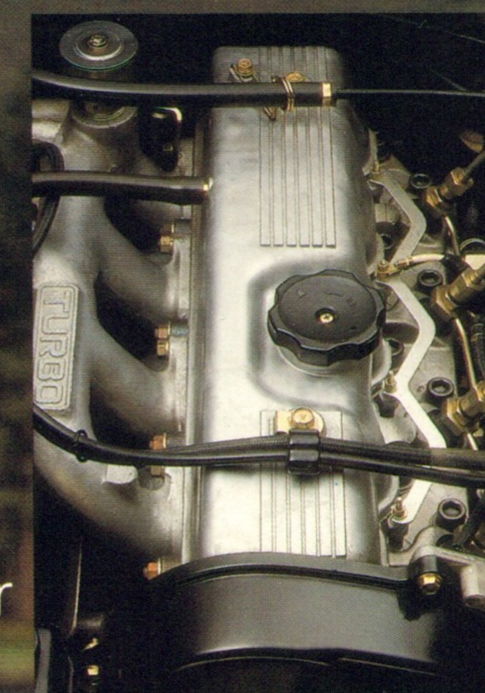
The ingenious Mitsubishi 2.3-liter Turbo Diesel engine.
