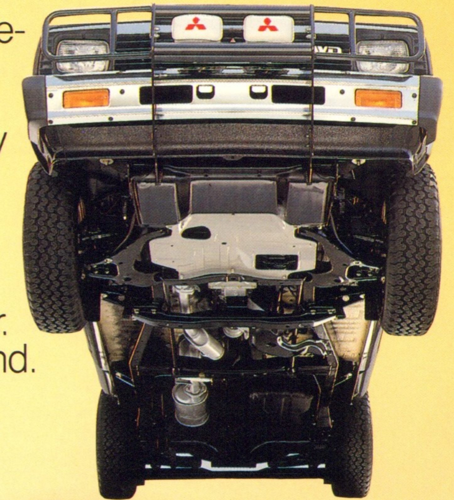
Every Mitsubishi truck is built on a rugged ladder-type frame with six major structural cross members.
