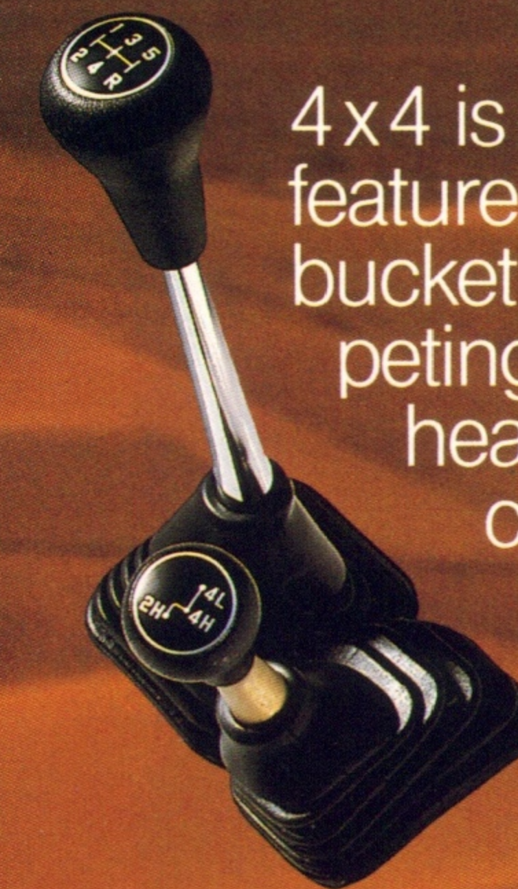
The integrated transmission and transfer case make for light weight and smooth shifts.
