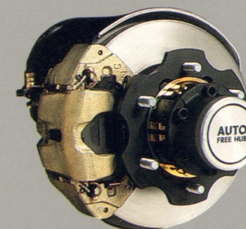
Big 10-inch power-assisted front discs are standard stoppers.
