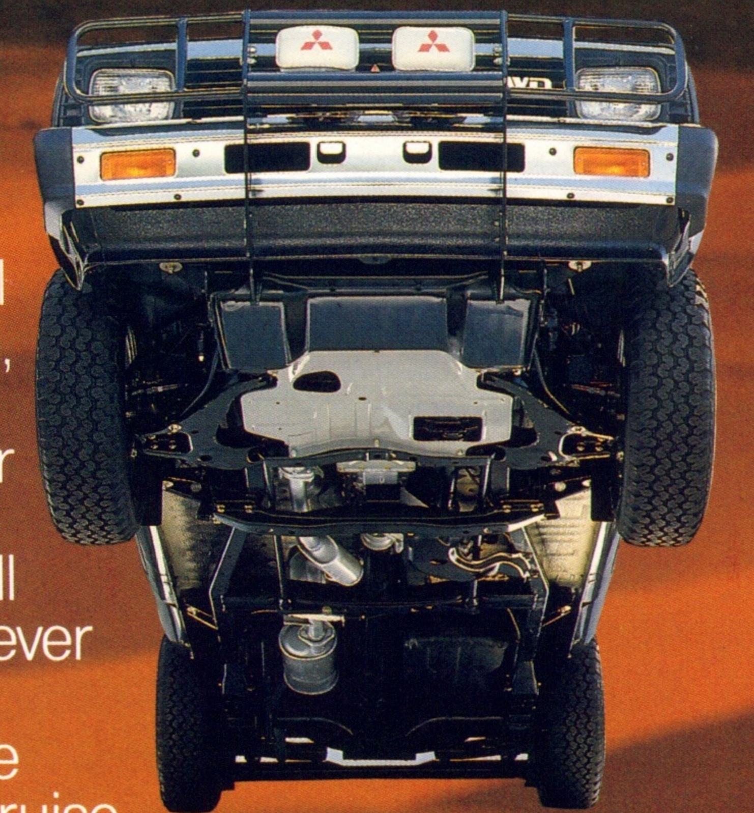
No less than six structural crossmembers add up to a strong, sturdy frame.
