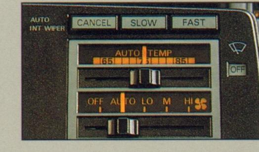
maintained automatically. But if you change your mind, controls for adjusting the air conditioner and heater are conveniently located behind the steering
