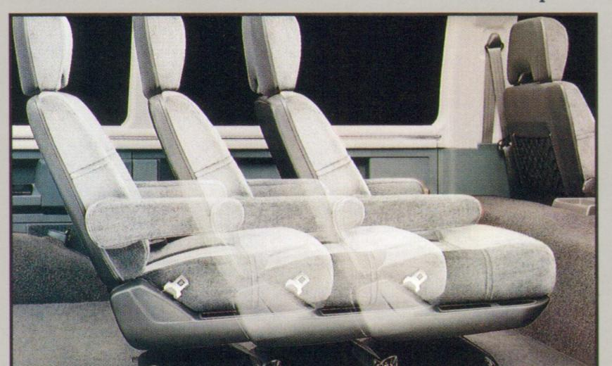
around. Our versatile seating system the rear bench seat. Slide it to full forward position. And you can haul a 1,576 pound payload in the standard Wagon.
