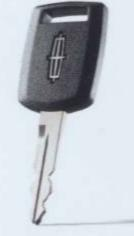
This is no ordinary key. This electronically coded ignition key is the hub of the Lincoln LS SecuriLock® passive anti-theft system. It prevents ignition bypass by allowing only the correctly coded key to start the vehicle. The security system is also armed once the key is removed from the ignition and disarmed only with the correctly coded key.
