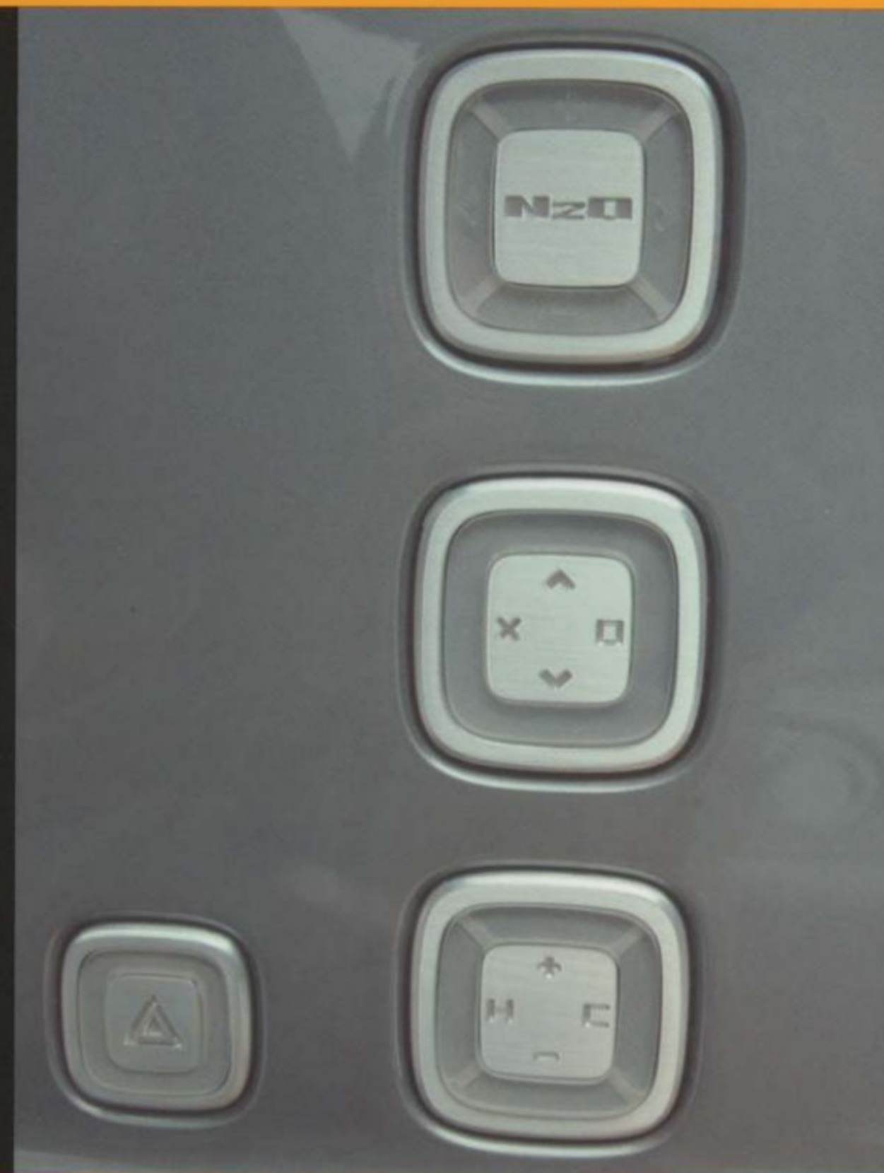
Interior controls are simple and functional. The top button delivers a performance-boosting shot of nitrous oxide.
