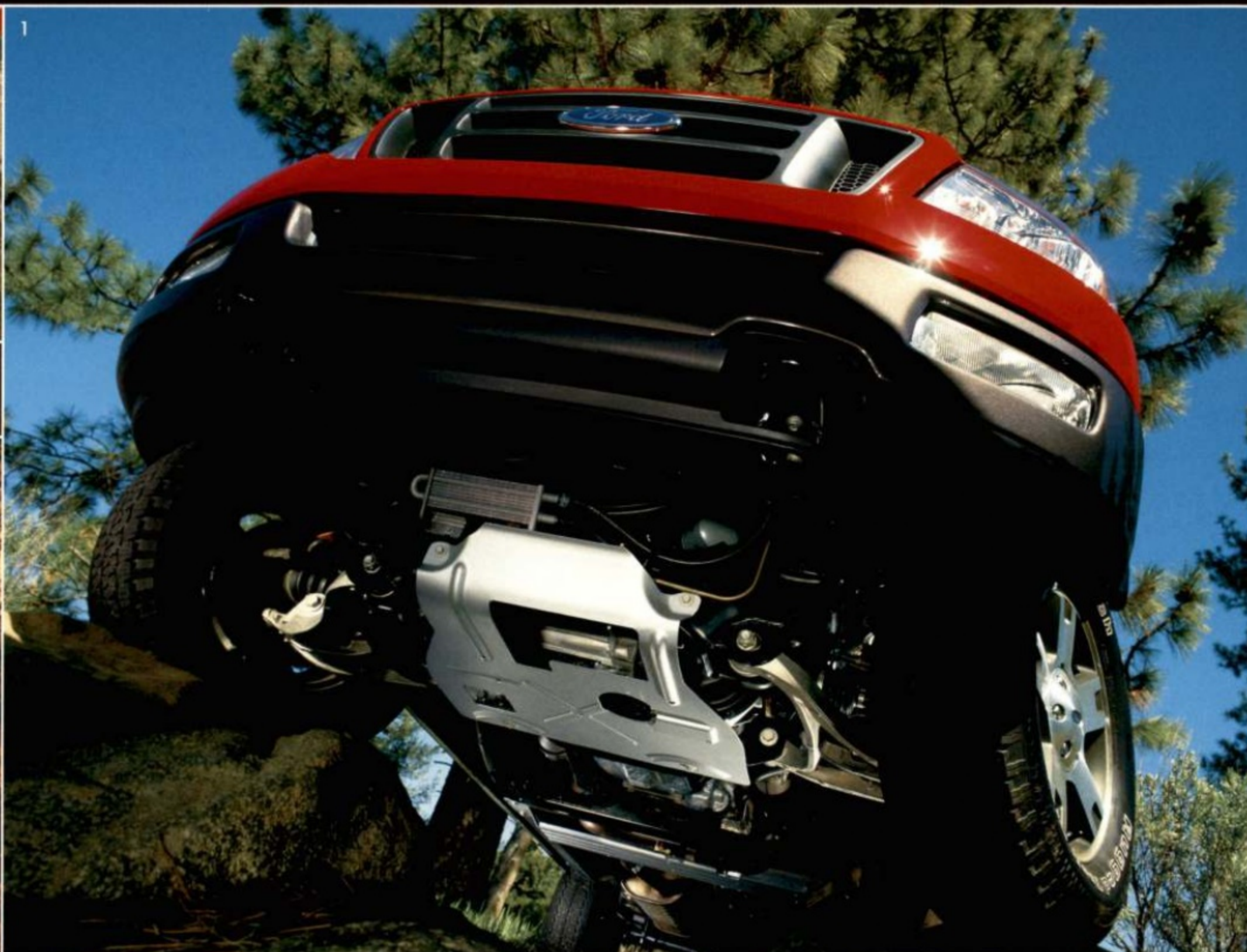
A rock's-eye view of FX4's skid plates, tow hooks and, though difficult to see, specially tuned off-road shocks. All able-bodied companions to the fully boxed frame and through-rail joint welds of the crossmembers.
