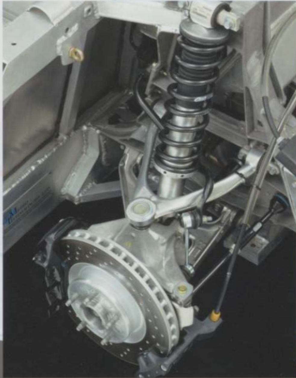
Rear shocks mount to a large, trellis-like aluminum structure that was developed for the Ford GT.
