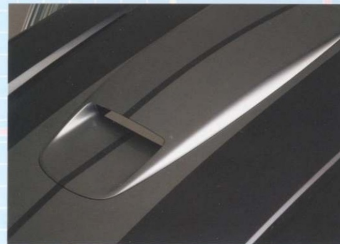
The low-rise hood scoop feeds air to a bank of 10 velocity stacks atop the mighty engine.
