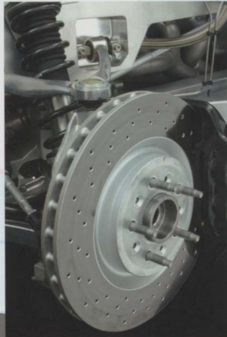
Brembo monoblock brake calipers and 14-inch front discs provide strong braking.
