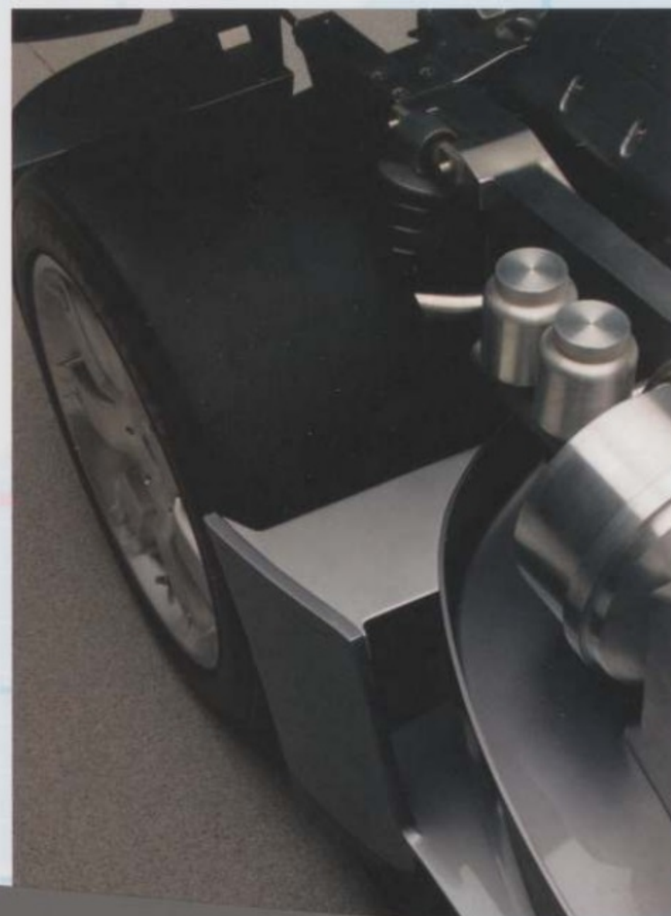
Every element shows its race-bred roots, including the Formula 1 – inspired barge boards that help channel hot air from the engine bay and front brakes.
