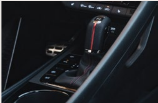
Available N 8-speed Dual Clutch Transmission (N DCT) The N DCT is an automated manual transmission with two separate clutches for increased efficiency, faster shifting and driving convenience.
