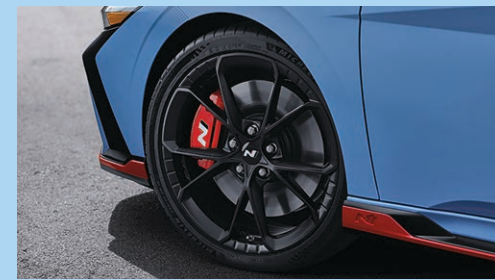
19" forged wheels and 14.2" front brake rotors
