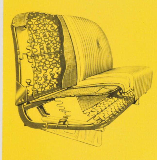
Meteor seats have special zig-zag springs which add to comfort and encourage correct, restful posture. Seats resist sagging . . . retain their shape and smart rounded contours.
