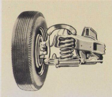
Suspension of each front wheel independent of the other means that a bump encountered by one wheel does not transmit a shock to the entire car. The shock is absorbed right there by "Hydra-Coil" springs and new "Oil-Cushion" shock absorbers mounted inside the coil.
