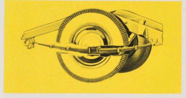
Rear spring suspension with two long, seven-leaf springs mounted parallel to the frame and the adoption of the new tension type shackle gives softer, freer spring action . . . greater riding comfort. Impregnated inserts and rubber bushings entirely eliminate the need for further lubrication.
