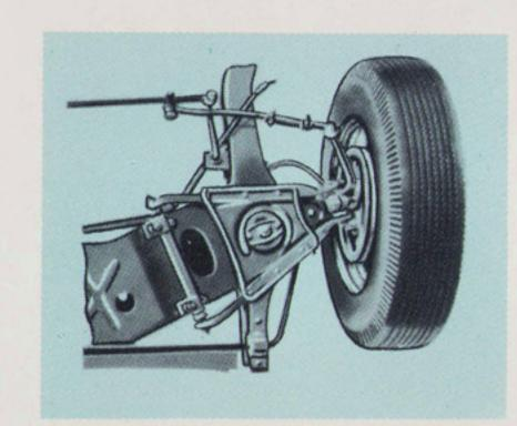
Straight-line steering on rough roads and in cross winds is made possible by Meteor's symmetrical steering linkage with Pitman arm and idler bracket . . . for maximum ease, safety and driver security.
