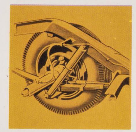
New "Oil-Cushion" shock absorbers, both front and rear, are hydraulic, telescopic and double acting. Refilling and adjustments are unnecessary because of permanent sealing.
