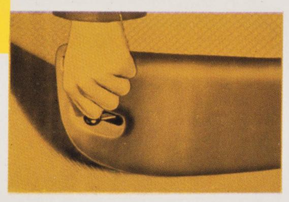
Front seat adjustment is easy, effortless with newly designed spring-actuated mechanism permitting 4½ inches total forward and backward movement. Seat tilts forward approximately ¾ inch... rises vertically ⅓ inch in extreme forward position for further support and comfort of shorter drivers.
