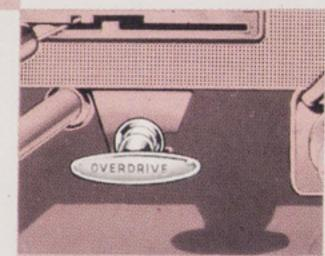
Meteor "Touch-O-Matic" Overdrive (optional at extra cost) provides an extra, economical forward speed cruising gear. Momentary release of the accelerator over 27 m.p.h. engages the Overdrive. Engine speed is then reduced 20% while car speed remains the same. Saves up to 15% in gasoline. Special 4.10 to 1 rear axle is used with Overdrive for better acceleration . . . greater hill climbing ability.
