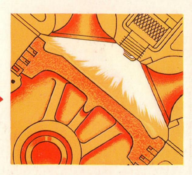
"Heart" of the great FireDome V-8 engine is the hemispherical, or "dome-shaped" combustion chamber. This has been proved the most efficient shape for complete combustion. There is less surface through which heat can be lost... more is converted into power. As fuel is burned more completely, there is less carbon deposit to reduce engine efficiency.
