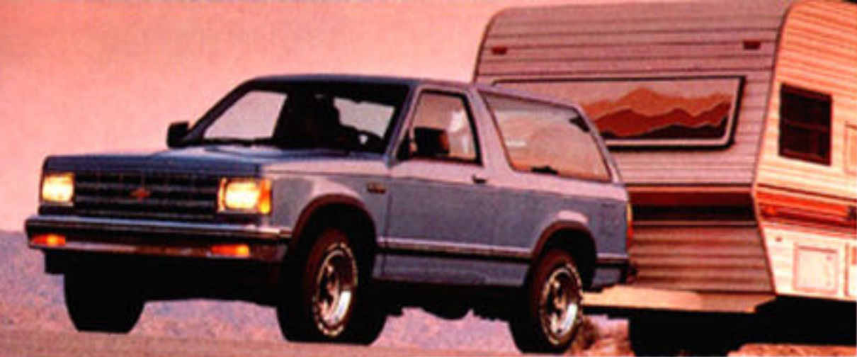
S-10 Blazer's available Heavy-Duty Trailering Package gives you 5,000 lbs. of towing capacity in the 2WD model, including trailer and cargo. (4,000-lb. capacity in the 4x4 model.)
