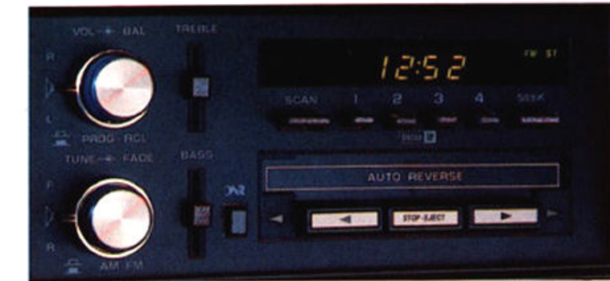
GM-Delco AM/FM stereo radio with cassette deck, seek and scan and digital clock.
