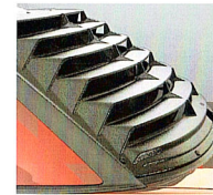
Rear louvre. Helps reduce glare and shades rear seat occupants.
