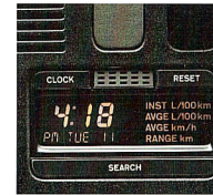
Trip computer. Displays fuel consumption, distance to empty and average speed.
