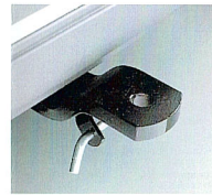
Tirebar (Class 1) Specially designed for Falcon. Tows up to 1200kg. Meets Australian Design Rule (ADR4-1) specifications.
