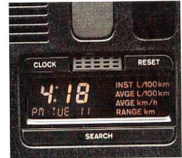
Trip computer. Displays fuel consumption, distance to empty and average speed.
