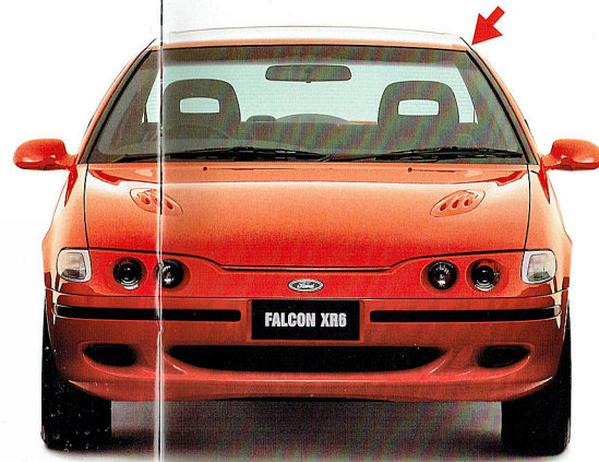
Falcons possess enormous roof crush strength. Ten new high strength steel structural reinforcements have been added to the body-side and roof structures. Falcon exceeds the standard US crush standard FMVSS 216 by 150% (best in its class).
