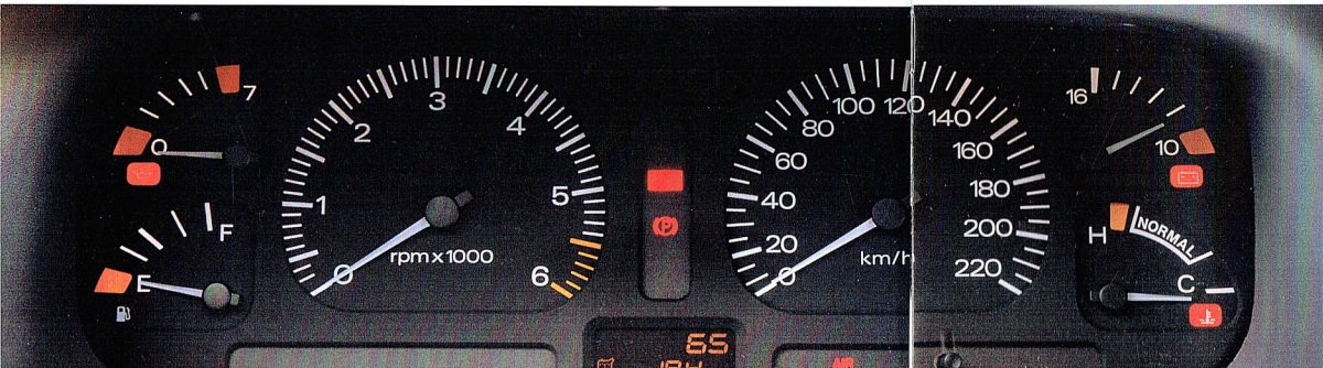
▶ The information centre – clear, clean XR Falcon instrument display feeds back vital data via tachometer, speedo, charge meter, fuel, oil pressure and temperature gauges.
