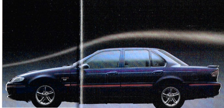
▲ Falcon's aerodynamic styling contributes to the overall efficiency of the vehicle. The air flow is directed over and around the vehicle to reduce drag. The resultant lower drag co-efficient combined with other engineering innovations and refinements help to promote efficient fuel usage.
