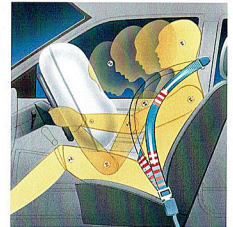
Belt locker device minimises payout of seat belt webbing under extreme conditions.
