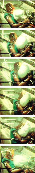
▲ The driver airbag is now standard on every XR Falcon model. Sensors in the vehicle detect the severity of an impact. If the collision meets the criteria for deployment, the airbag will inflate and be released to help protect the driver. All this occurs in less than one twentieth of a second.
