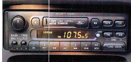
▶ The XR Falcon quality 6-speaker 60 watt audio system incorporates numerous features for your convenience and listening pleasure including soft touch controls, tape hold during radio listening and keyless play.
