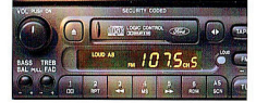
The vehicle's audio system is protected by another Ford anti-theft measure. A special security code renders the unit useless to thieves.
