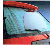
▲ If reverse gear is selected when the front wipers are operating, the rear window wiper is automatically activated.
