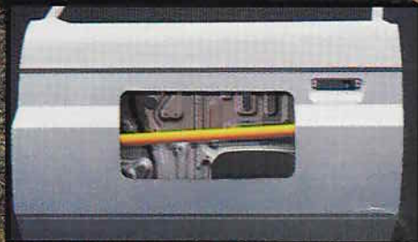
Side intrusion beams are fitted in the doors.
