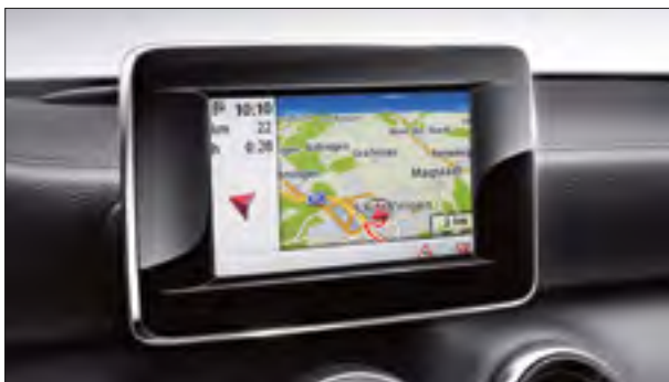
The Becker® Map Pilot navigation system works with the Audio 20 radio/single CD's display and the multi-function display in the instrument cluster
