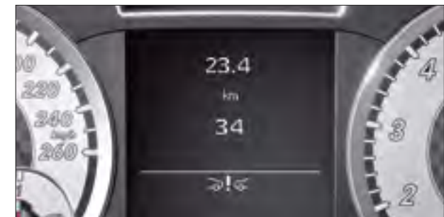
Collision Prevention Assist can warn you if it detects you come too close to the vehicle or object in front
