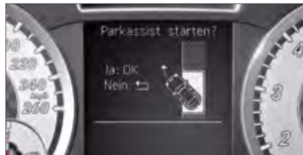
Active Park Assist displays the status of the parking manoeuvre in the instrument panel
