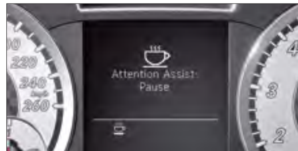
If it detects signs of tiredness or inattentiveness, Attention Assist recommends taking a break
