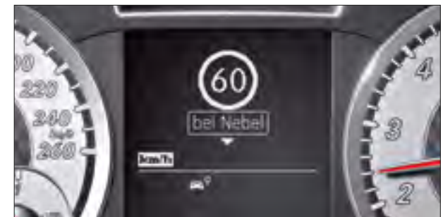
Speed Limit Assist shows the permitted maximum speed in the instrument panel and on the COMAND Online display
