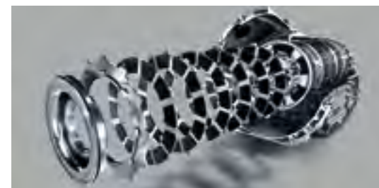
AMG Speedshift MCT 7-speed sport transmission
