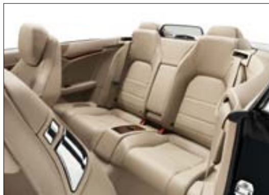
To ensure even those in the rear can enjoy unruffled open-top motoring, the windshield helps reduce interior air turbulence as part of the Aircap system
