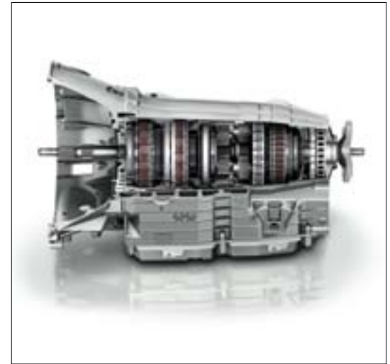
7G-Tronic Plus can skip gears in downshifts for more rapid acceleration
