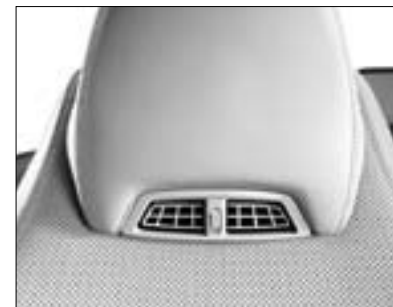
Aircarf neck-level heating system for Cabriolet
