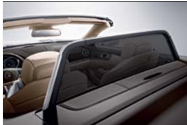
The electric wind deflector keeps draughts to a minimum in open-top driving
