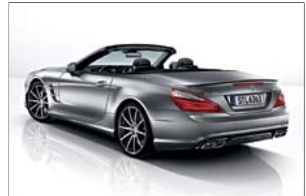
AMG sports exhaust system with two sets of twin chromed tailpipes
