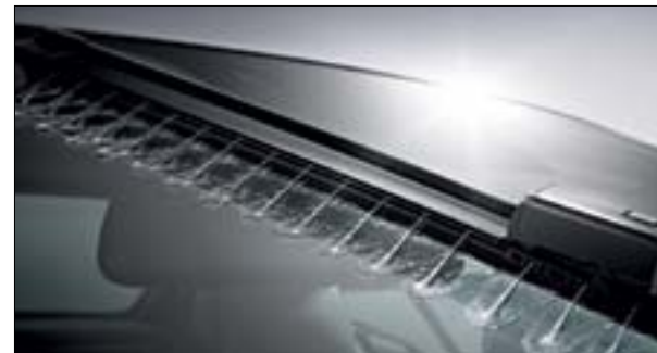
Magic Vision Control: the SL's adaptive windscreen wash system cleans the windscreen without impeding visibility
