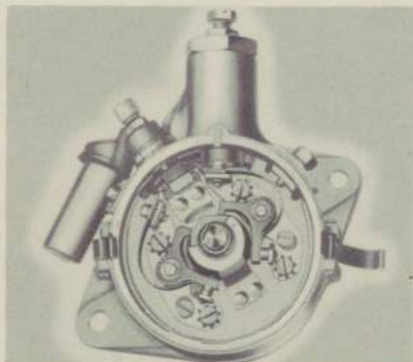
The Ford sealed-dry distributor on the V-8 has two sets of points for greater reliability, supplies hotter sparks for better performance.
