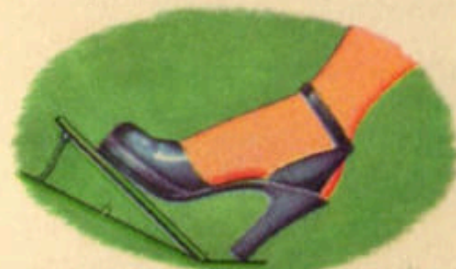
Pressing accelerator all-the-way down returns car to direct drive.
