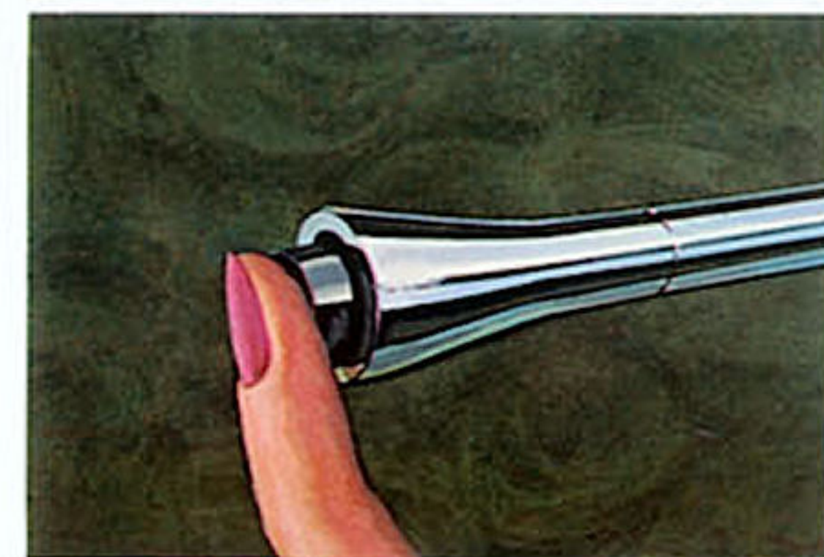
Fingertip Speed Control. Button on end of turn signal lever actuates automatic control to permit travel at desired speed with your foot off the accelerator pedal. Touch the brake and control returns to driver. (V-8 and SelectShift required.)
