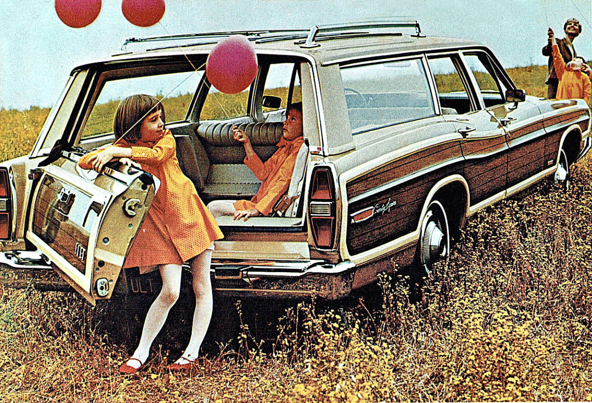
Magic Doorgate. Ingenious hinge design lets you swing Doorgate out like a door for passengers, or down like a tailgate for cargo. Standard on all Ford station wagons.
