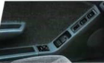
Power window and power door lock controls are conveniently located on the XT6 driver's side door panel.
