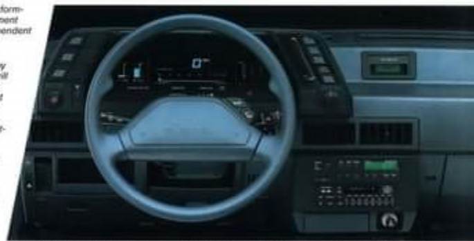
Advanced GL-10 digital instrument panel includes graphic tachometer, turbo boost indicator, 7-function trip computer, and 20-watt ETR AM/FM stereo. Shown with optional ED cassette deck.
