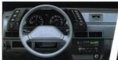
Quick reading among instrumentation of the GL Sedan includes tachometer, voltmeter, oil pressure gauge, and 10-watt ETR AM/FM stereo. Shown with optional Elite cassette deck.
