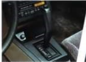
Optional computer-controlled 4-speed electronic automatic transmission.
