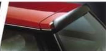
Rear dust deflector helps keep rear window clean.
