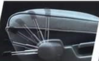
Driver's seat height adjustment, together with adjustable lumbar support, lets you set your optimum driving position.
