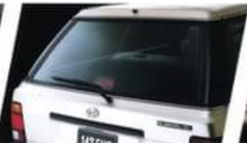
Rear window wiper/washer with electric defogger provides excellent all-weather visibility.
