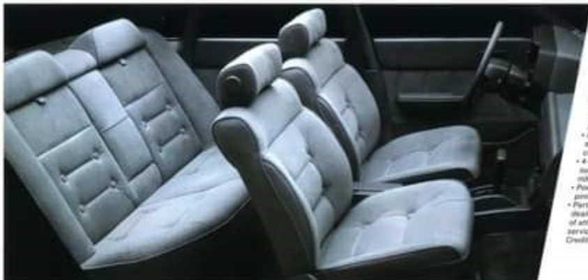
Graceous, luxurious GL-10 interior with suede-like cloth upholstery. Fully reclining front bucket seats feature driver's seat height adjustment. Rear seat features 2-way folding seatback with trunk-through feature.
