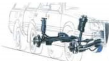
Electronic air suspension for "ride-on-air" comfort, standard on the GL-10 Full-Time 4WD Turbo Wagon.
