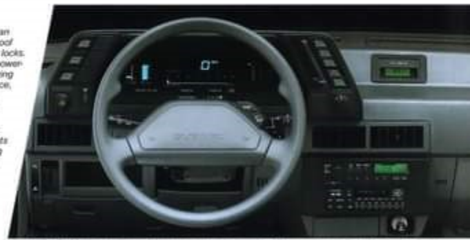
State-of-the-art GL-10 digital instrument panel with graphic tachometer, 7-function trip computer, and 20-watt ETR stereo system. Shown with optional EQ cassette deck.
