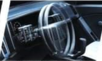
Telescoping-tilt steering wheel, 4-in. control posts and instrument panel for optimum driving convenience and comfort.
