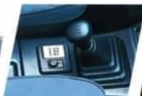
GL-10 Full-Time 4WD Turbo features 5-speed transmission with center differential locking switch for maximum traction.
