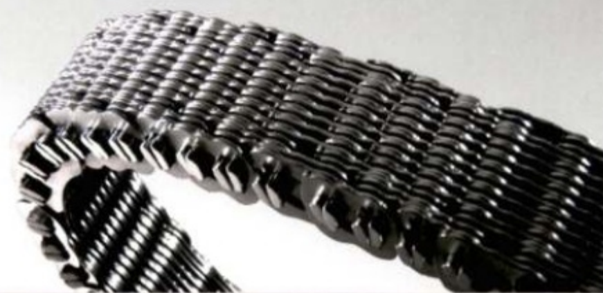
CVT's Steel-Link Belt
