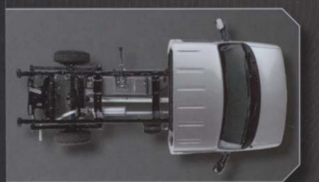
NEW E-250 SUPER DUTY® CUTAWAY — Yet another model to help you get the right vehicle for your needs. This segment-exclusive configuration offers an 8600-lb. GVWR and a 4370-lb. payload. Its 4.6L Triton® V8 and 4-speed automatic transmission are standard.
