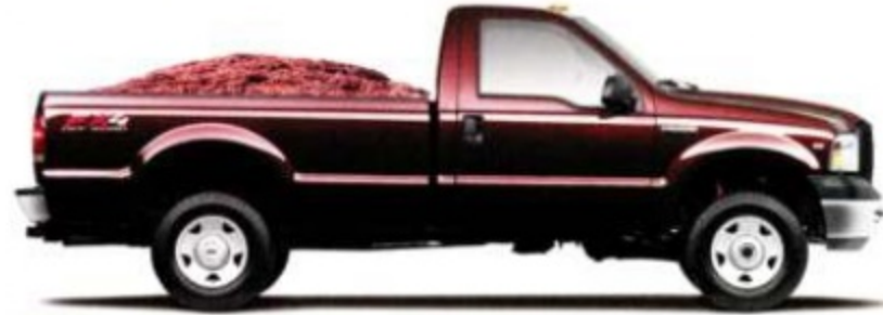
REGULAR CAB: MAX. PAYLOAD F-350 SRW – Max. 4400 lbs. F-350 DRW – Max. 5800 lbs.
