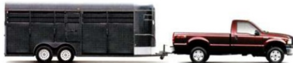
REGULAR CAB: MAX. CONVENTIONAL/MAX. 5TH-WHEEL TOWING F-250/F-350 SRW – 12,500/17,000 lbs. 1 F-350 DRW – 15,000/19,200 lbs.
