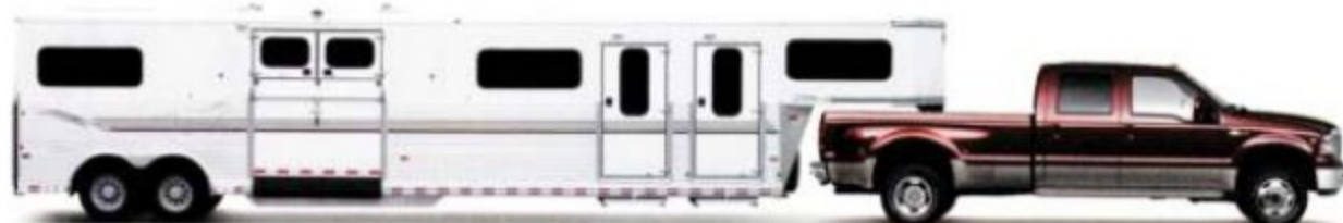
CREW CAB: MAX. CONVENTIONAL/MAX. 5TH-WHEEL TOWING F-250/F-350 SRW – 12,500/16,500 lbs. F-350 DRW – 15,000/18,600 lbs.
