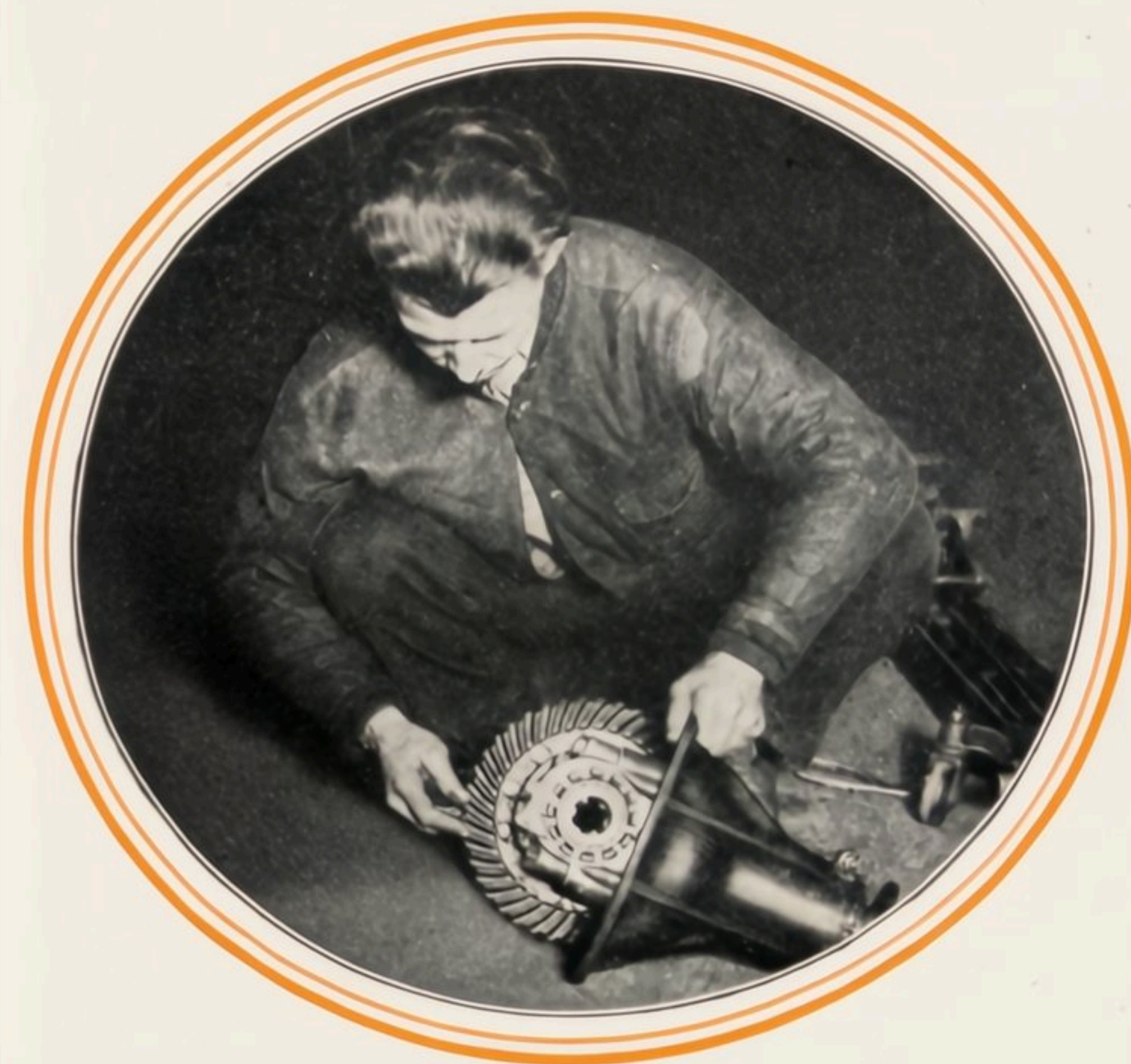
Member of A.A.A. technical committee counting number of teeth in differential and pinion gears to prove that only stock gear ratios were used in the three Studebakers which set new world records for speed and endurance
