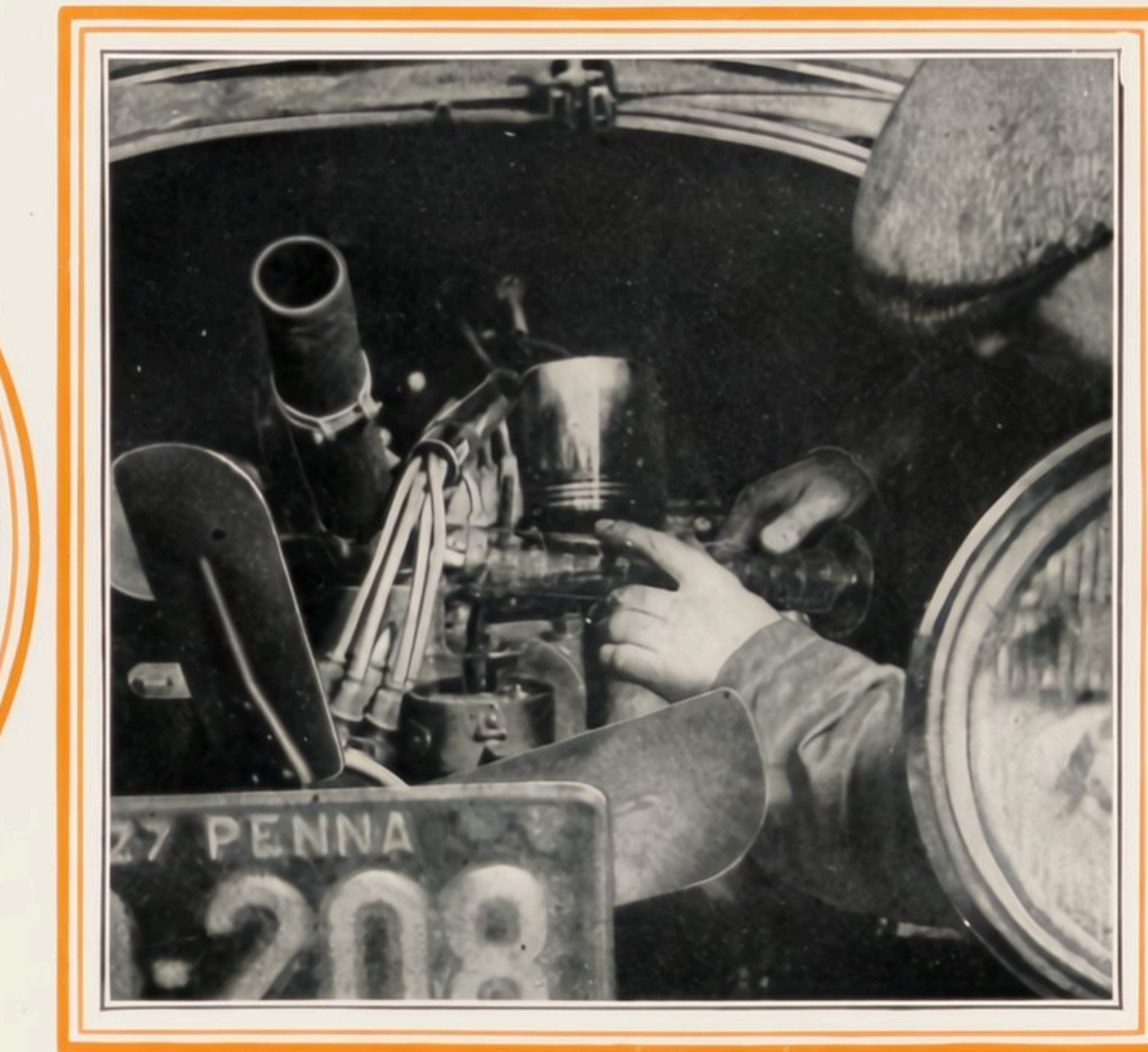
Nothing was left to doubt. Here you see an official of the American Automobile Association checking compression ratio on Commander model selected at random from dealers' stock—to compare with 25,000-mile Commanders
