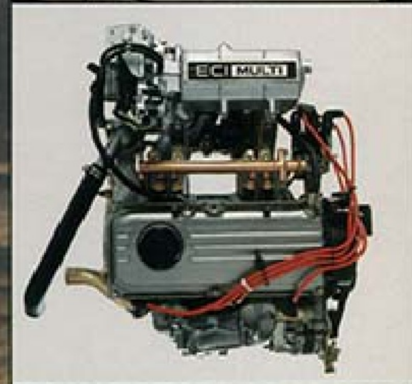
1.5 liter multi-point electronically fuel-injected engine
