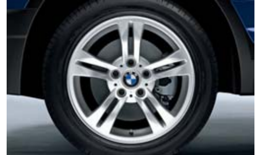
■ 17 x 8.0 Double Spoke (Styling 112) alloy wheels and 235/55R-17 all-season tires are standard on the X3 3.0i.
