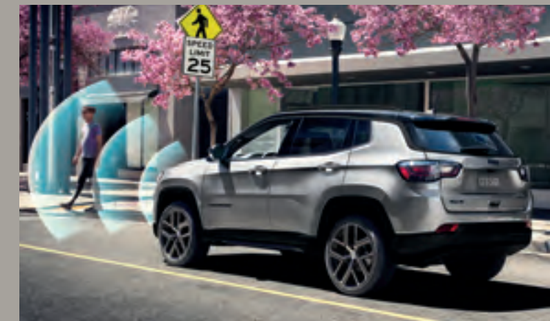
PEDESTRIAN / CYCLIST EMERGENCY BRAKING 14 Drivers are provided a warning and the vehicle automatically decelerates to help avoid an impending collision with a pedestrian or cyclist ahead. Standard.
