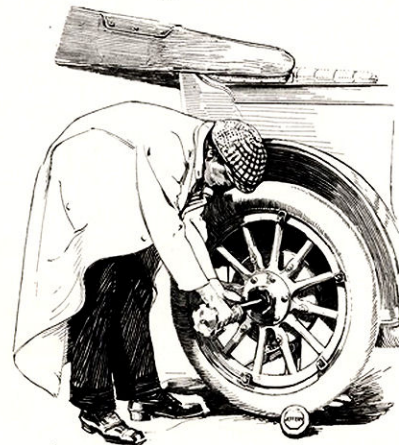
Removing drive shaft from Jeffery full floating rear axle
