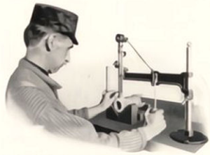
Delicate device for testing Jeffery gears with hair breadth accuracy
