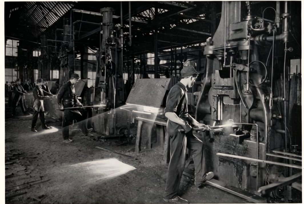
The Jeffery drop forge shop, where all drop forged parts for Jeffery cars are made
