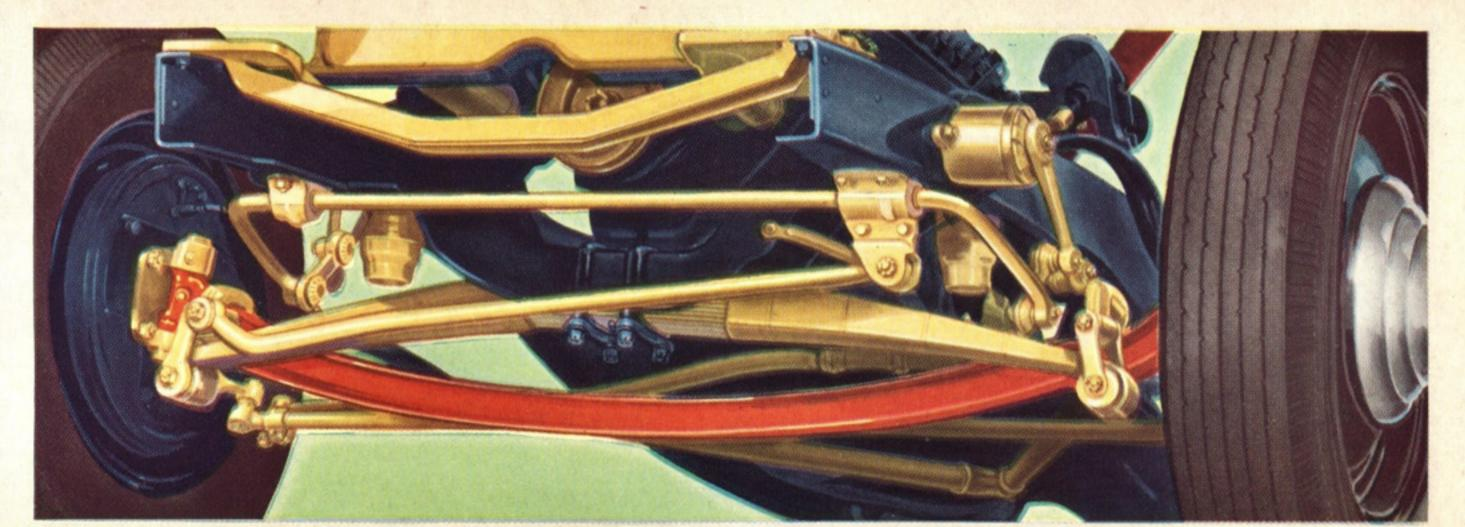
DOUBLE-ACTING hydraulic shock absorbers are of an improved design this year, for maximum riding comfort. Mercury springs, front and rear, are increased
