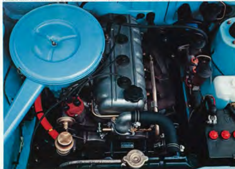
102hp, 1600cc engine with higher performance 2-barrel carburetor
