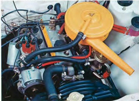
1.6L engine with 5 main bearings, not 3
