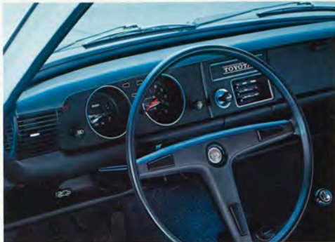
Padded dash with recessed, glow-panel instrument panel (Photo: Seiden and Watson)
