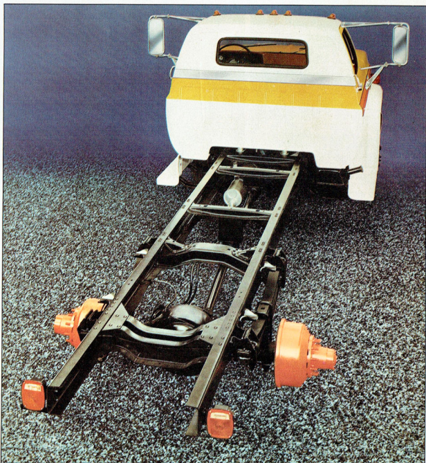
Vacuum/Hydraulic brakes are standard on some models depending on GVWR and GCWR ratings. They feature a dash-mounted master cylinder and frame-mounted vacuum booster.
