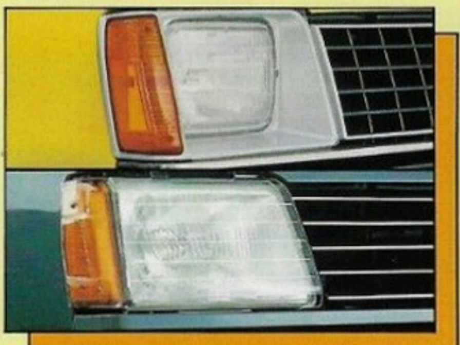
HEADLAMP GUARDS. Moulded plastic style that enhances appearance and protects against accidental headlamp damage. Removable for easy cleaning of headlamps.
