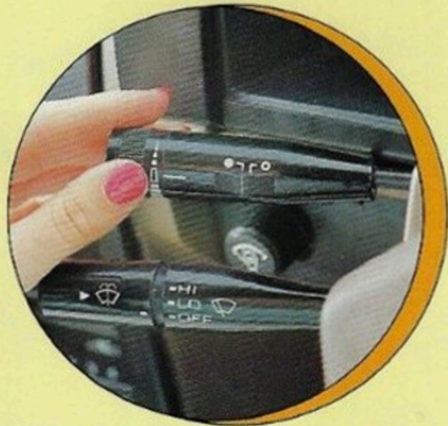
CRUISE CONTROL. Graduated, easy-to-read speed set dial to enable cruising speed to be pre-set. (Speed can be changed whilst cruising.) Does not require speed reset after every stop. Steering column mounted to complement vehicle interior.
