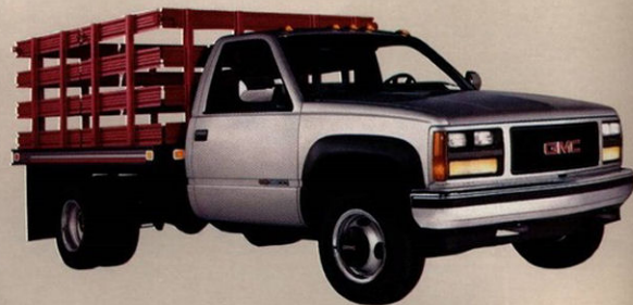
4-WD Sierra SLX Series 3500 Cab & Chassis and available dual rear wheels features an available stake rack body (1)
