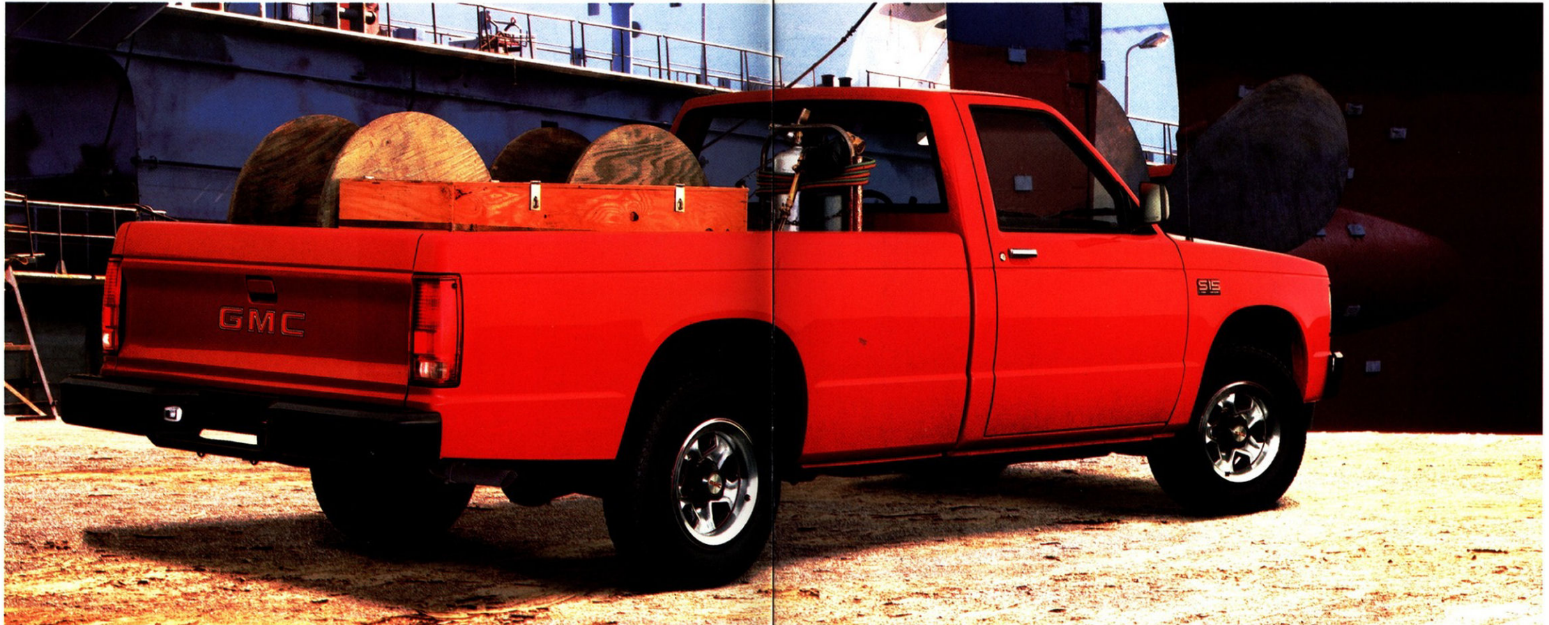
8 S-15 Pickup's cargo box sides and tailgate utilize tough, double-wall steel construction. Built-in eyes at each corner permit cargo tie-down.
