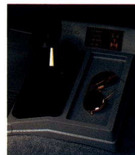
Single-lever Insta-Trac transfer case control allows you to shift from 2-WD to 4-WD HIGH and back, at any speed. A lighted display indicates your driving mode.
