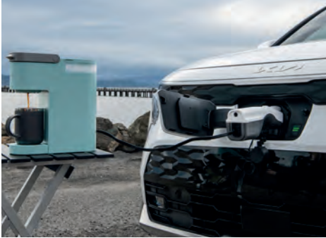
The Vehicle-to-Load feature turns your Niro EV into a 120V AC power source*
