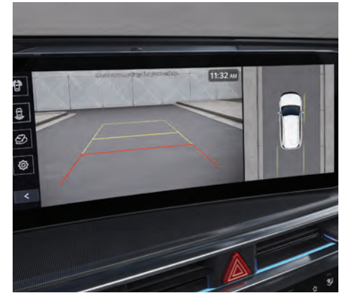
The Surround View Monitor displays the situation around your vehicle to assist you with safe parking.*
