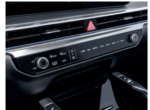
Infotainment/climate switchable controller share the same LCD softkey keyboard.
