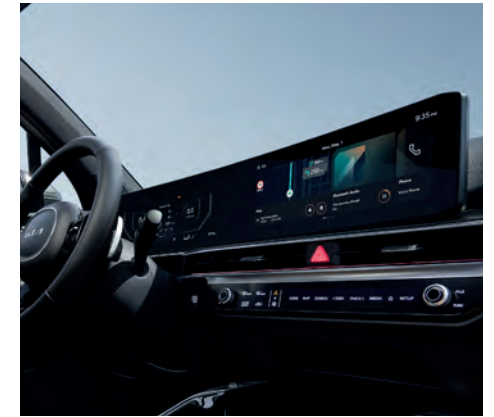
The panoramic curved display combines driving functions and the centre 12.3" infotainment screens in one manageable frame.
